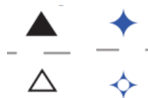
Figure 8. Chart symbols for Fixes (black and hollow triangles) and Waypoints (blue and hollow 4-point star). (Aeronautical Information Services - Aeronautical Chart Users' Guide, FAA)
