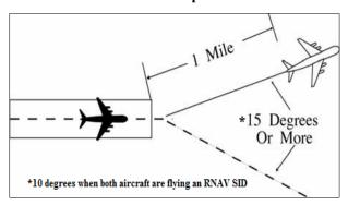
FIG 5-8-2 Simultaneous Departures
