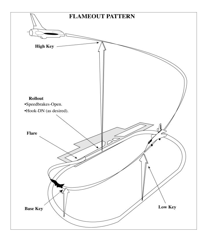
FIG 3-10-15 Simulated Flameout [2]
