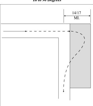
FIG 6-5-5 Overflown Side Minima 16 to 90 Degrees
