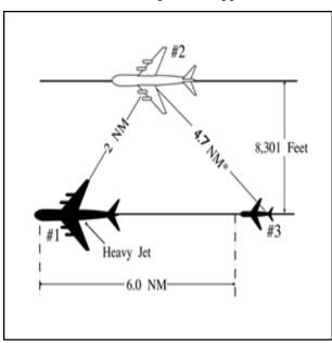
FIG 5-9-6 Simultaneous Dependent Approaches
