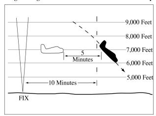
FIG 6-4-10 Climbing Through Another Aircraft's Altitude Timed Separation
